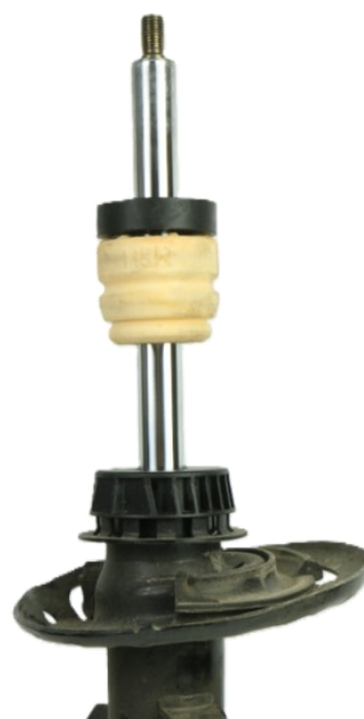
Fig. 1: Bump rubber and rubber spacer
