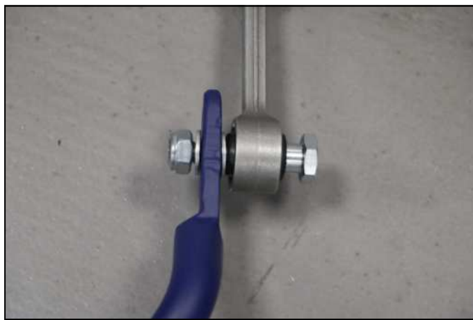
Fig. 2: Tightening of the screw with approx. 50 Nm
