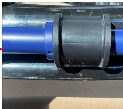
Fig. 2: Mounting of the Anti-Roll Bar ends
