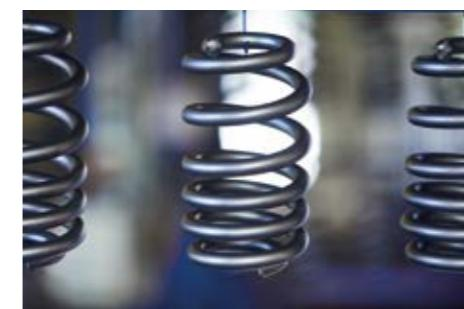
Surface treatment: Internally: In-house, powerful system for zinc-phosphatizing as well as epoxy resin and polyester coatings in all the common RAL colours. Externally: We offer any commercially-available surface treatment desired.
